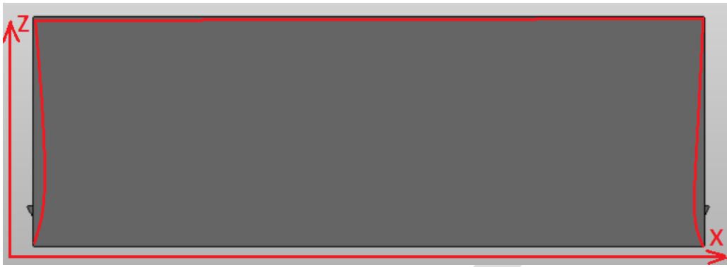
Figure 6 Part with detents on the side walls helping to measure the distortion
