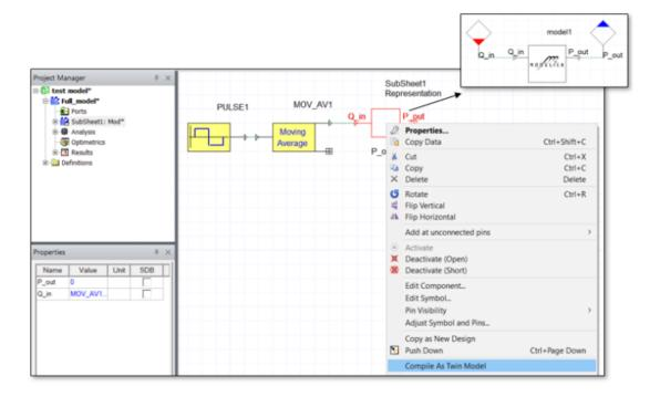
Once the Twin Model is created, it can be exported as a Fluent Component by right-clicking on the corresponding model name in the Definitions -> Models item in the Project Manager, as illustrated below. A file with the .flsimextension will be created on disk.
